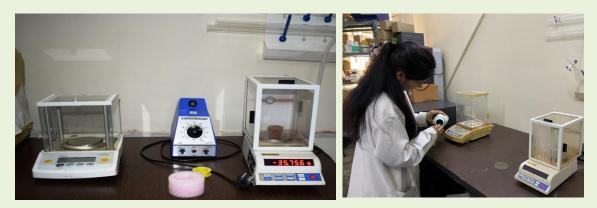
> These balances are used for weighing of compounds with 0.0001 gm accuracy.
